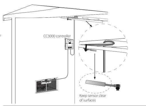
Connect the room temperature sensor to green connector J11 Pin No: 1 and 2
